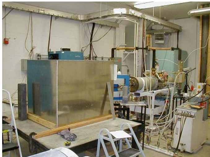
Figure 4. The 30-MeV Electron Linac. Peak performance is achieved at 25 MeV. In addition, peak power occurs at less than the maximum energy, so that the accelerator is currently operated at 20 to 25 MeV. The tank and stand are also visible.
