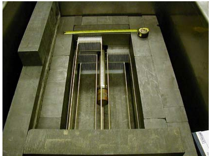
Figure 6. RACE Fuel Trays and Target Inside the Graphite Reflector
